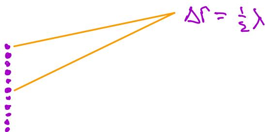
so right next to 1<sup>st</sup> max we will fall quickly to zero amplitude due to all the cancellations
