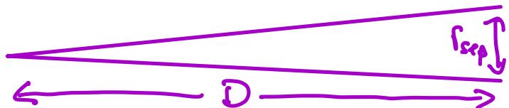
$$\Theta_{\text{sep}} = \frac{r_{\text{sep}}}{d} = \frac{1.22\lambda}{D} \quad D = 4 \text{ mm eye pupil}$$
