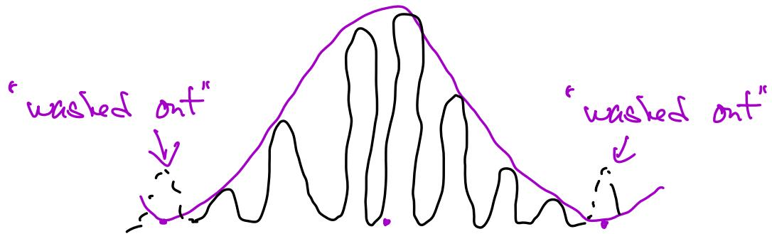
⇒ in general, if interference maxima between diffraction minima will be
