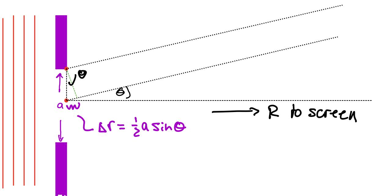
4. These 2 rays will cause destructive interference at the point on screen that is at  $\Theta$  (with respect to horizontal) if path difference is  $\Delta r = \frac{1}{2}\lambda$
