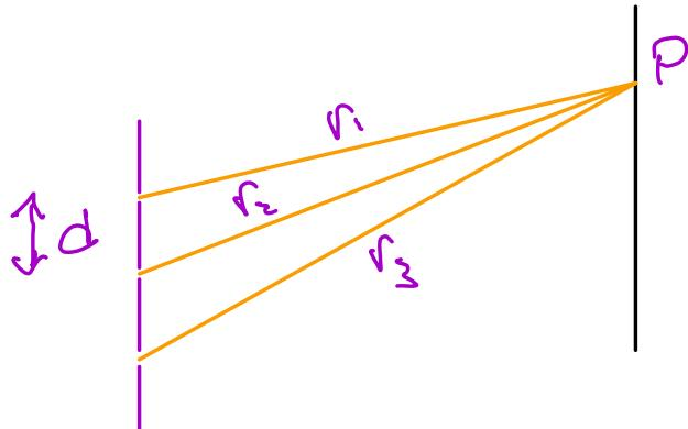
this wave will also add constructively at  $P$  because the path diff to the other 2 waves will also be a multiple of  $\lambda$
